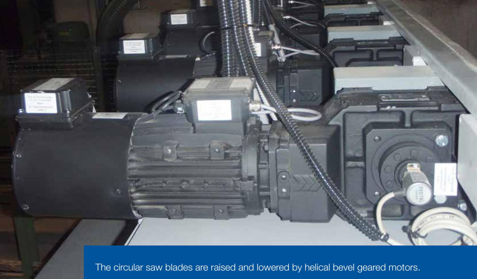
The circular saw blades are raised and lowered by helical bevel geared motors.
