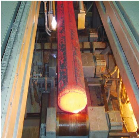
Picture 1: Conveyor line of a continuous casting plant with WATT roller table motors
