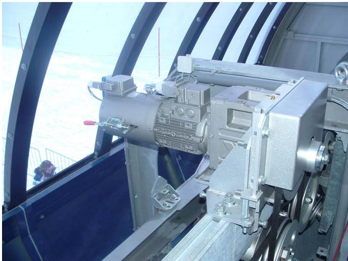
Figure 3: WATT helical geared motor with motor modules
