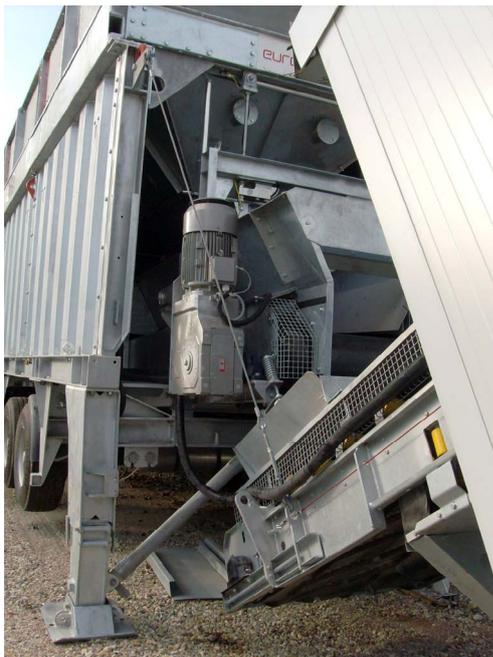
Figure 1: Bunker unit with conveyor belts
