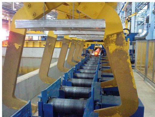
Picture 1: Dip tank manipulator
