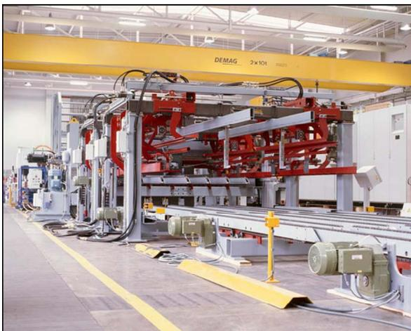
Figure 1: ATT type industrial mesh welding system
