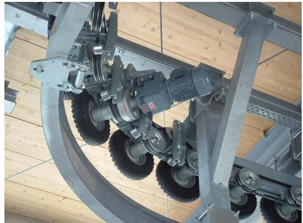
Figure 2: Roadway with Watt helical gear motor
