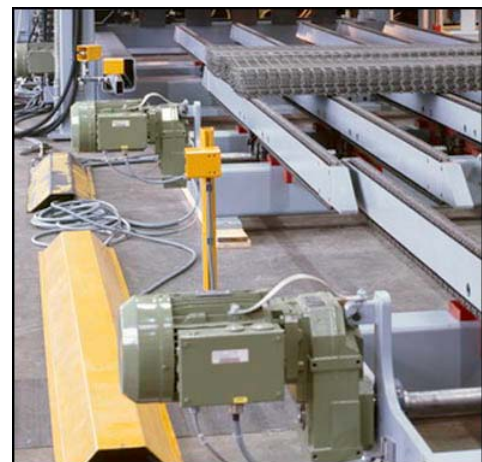
Figure 2: Shaft mounted geared motor ASA 66A 114M4 TH with MIP box
