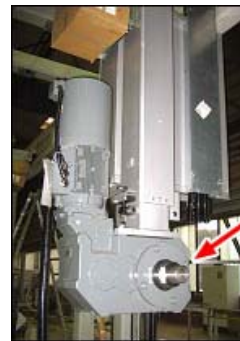
Fig. 2: Winder drive unit KK 136A 161L4 BR150 IG FLTH
