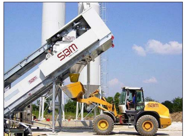
Figure 2: Concrete removal on the EUROMIX 1000/1600
