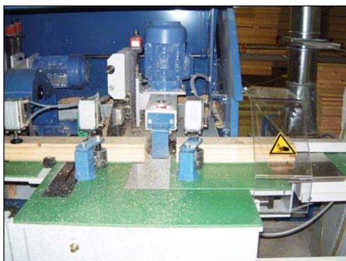
Fig. 1: Face groove cutter with WAC 101L2 TH (3kW)
