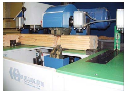
Fig. 2: 4-way milling machine with drive motors (3 or 4kW)
