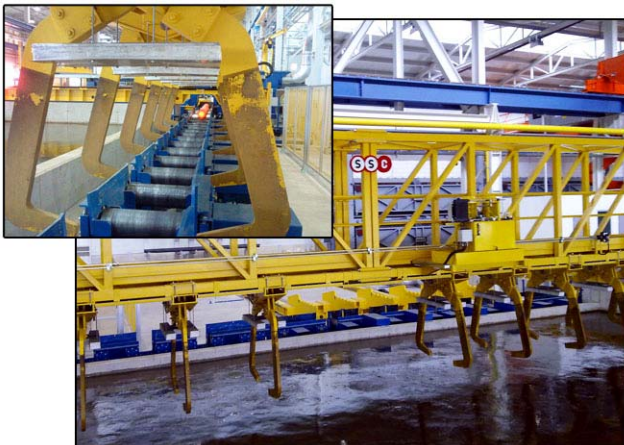
Picture 1: Dip tank manipulator
