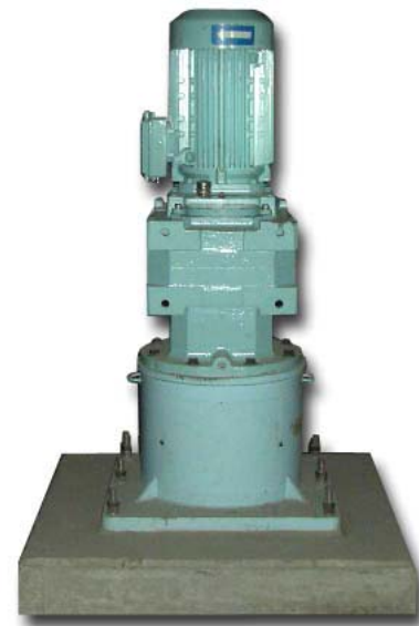
Picture. 1: Vertical mounted agitator gearbox FRA 130A 160M4
